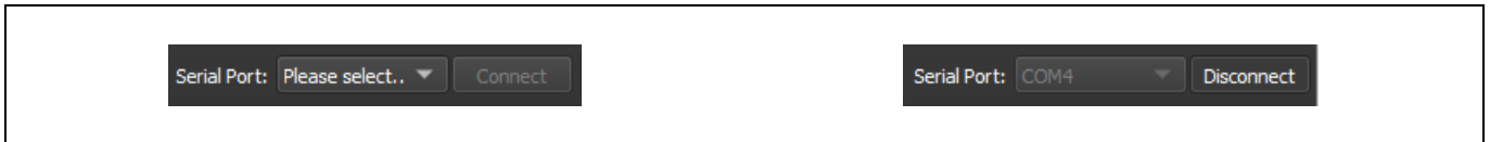
Figure 5 Serial Port Connection: Not Connected (Left), Connected (Right)
